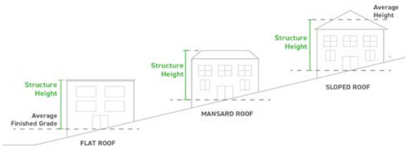
Illustration of how to measure building height
