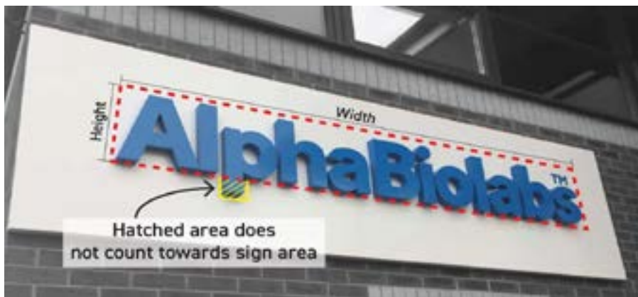
Illustration of letter descenders that are not counted toward wall sign area
